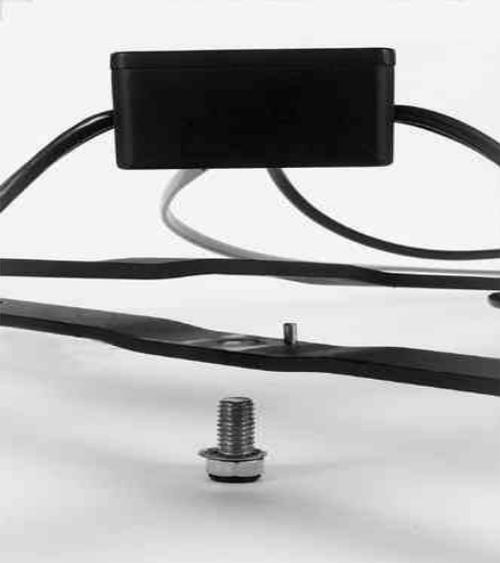
The initial assemble begins by aligning the two pieces of flat stock. These are placed together to form an “X”. Use the guide pins to align the two pieces of the “X” arm ( visible in Figure 5). The pin should extend through the overlapping cross arm.
