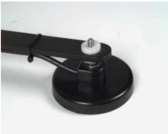
The small end of the plastic spacer should be facing down. This will have the small end of both plastic spacers inside the hole. By doing this, you are assured that the Antenna Whip will make a proper electrical contact to the cables, but will not be grounded against the “X” arms ( Figure 17 ).
