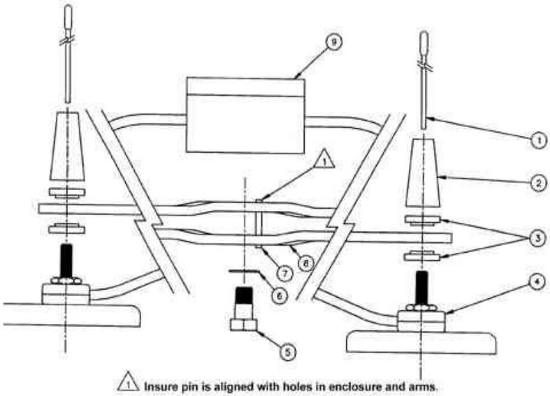
Figure 4 shows the DFjr antenna assembly as an exploded view of the major components.
